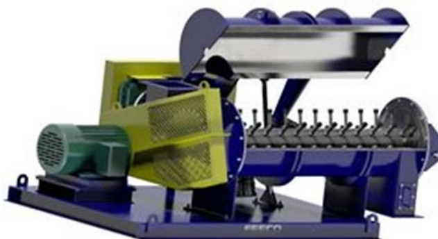
Figure 5.1.1 Industrial pin mixer for carbon black pelletizing 27 .
