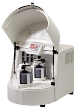
Figure 3 Planetary ball mill used for grinding and pelletizing. Model: Pulverisette 5/2 by Fritsch.
