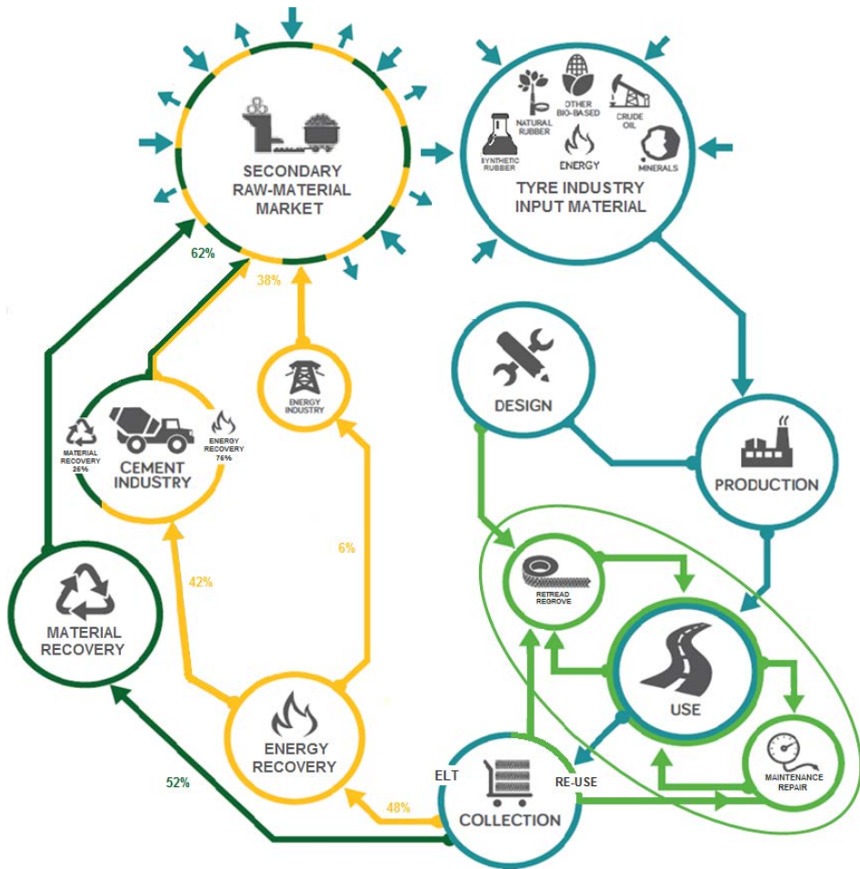
Figure 2.2 Tire life cycle with various recycling loops 5 .
