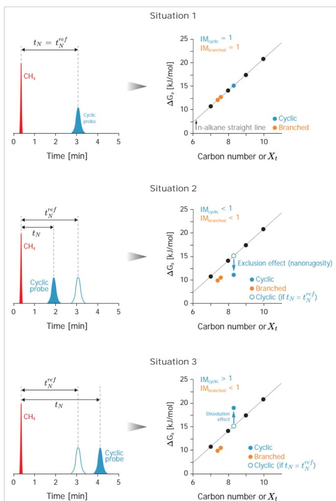
**Figure 1** - Schematic GC chromatogram (left) and variation of free energy change of adsorption ( $\Delta G_a$ ) of n-alkanes, branched and cyclic probes as a function of their corresponding carbon atom number or Wiener topology index ( $X_t$ ) (right).
