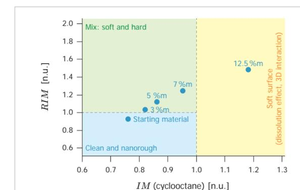
**Figure 3** - Evolution of the surface behaviours with the grafting ratio.
